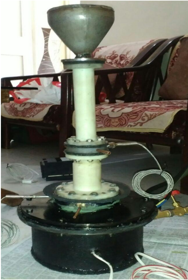
Fig 28 : Assembly of Thermoacoustic refrigeration system
