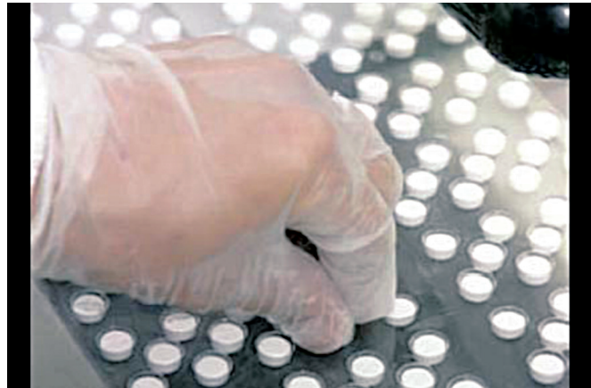
Figure 4: Blister packing process needs low temperature and humidity
