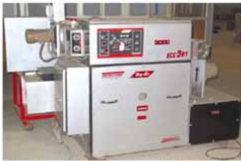
Figure 8 : Rotating Honeycomb dehumidifier
