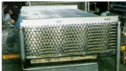
Stainless Steel Blast Freezer coil for use with Ammonia
