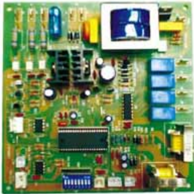
Figure 6: Typical electronic controller
