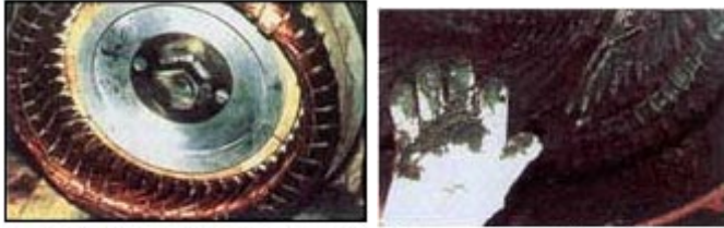
Motor stator before burnout Motor stator after burnout
