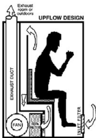
Figure 5a : Sputum induction chamber : Upflow design
