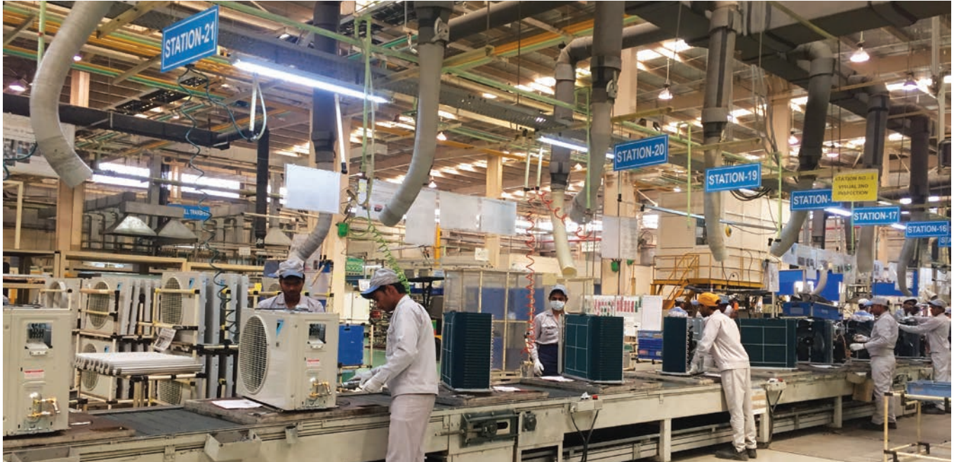
An air conditioner ODU assembly line
