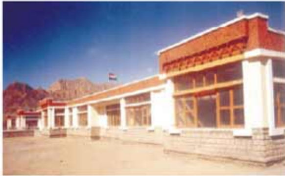
Large south-facing windows for solar gain in cold climate of Leh.
