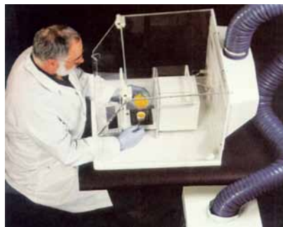
Photo 3 : Ventilated cabinet for carrying out weighing operations.
