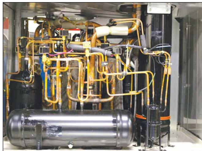
Chart 5 : DC rotary inverter system mechanical architecture.
