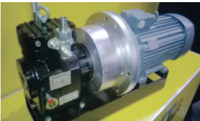
Photo 13: 7 kW ammonia reciprocating compressor
