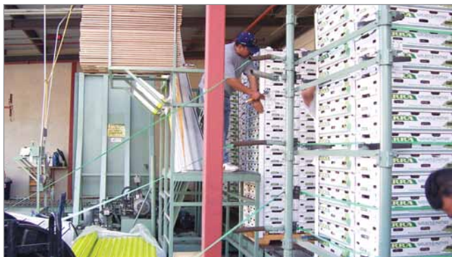
Photo 6 : Conveyor for pallets with strapping mechanism
