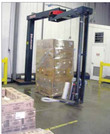
Photo 8 : Automatic wrapping machine. The arm with the film goes around the pallet with the film roll moving downwards
