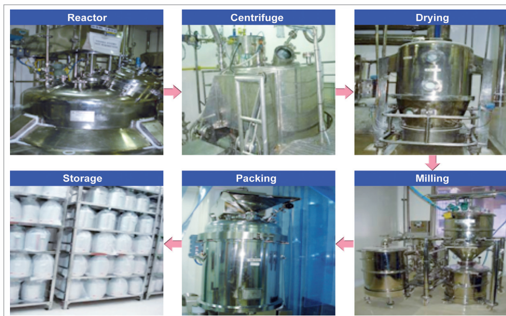
Figure 3: API manufacturing process flow diagram
