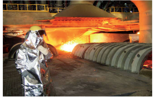
Figure 9: Forced ventilation and fume extraction of cast house
