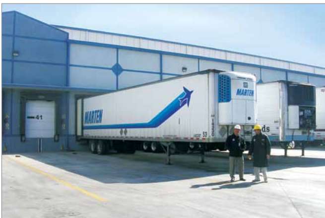
Photo 19 : Container docked without the driving unit with only the condensing unit
