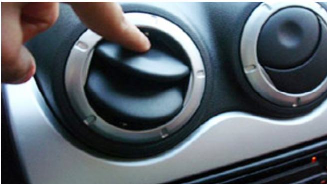
Figure 4: Louvres in the air outlet
