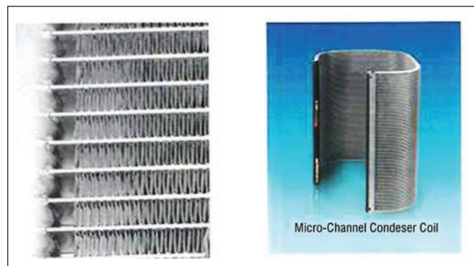
Figure 5: Life of micro channel coil shortened by crude maintenance practices
