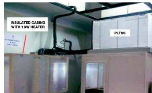
Figure 4: Test Rig of PLTSS with PCM 25
