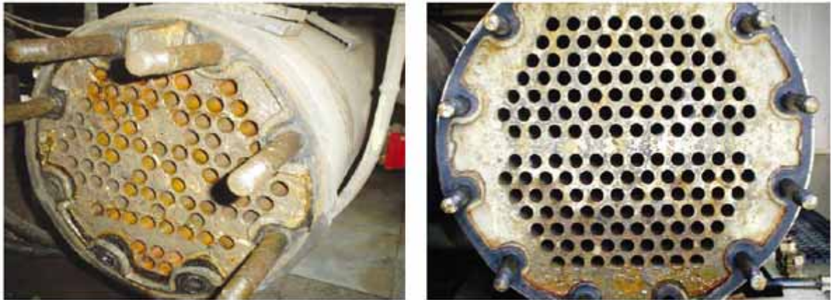
Comparison of condenser tubes in a chiller package treated with chemicals (left) and ULF (right). Photo courtesy of Technova Imaging Systems (P) Ltd.
