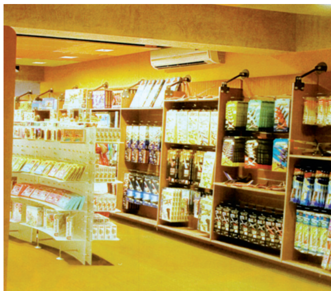
An air conditioned hobby store with a non-ducted split AC
