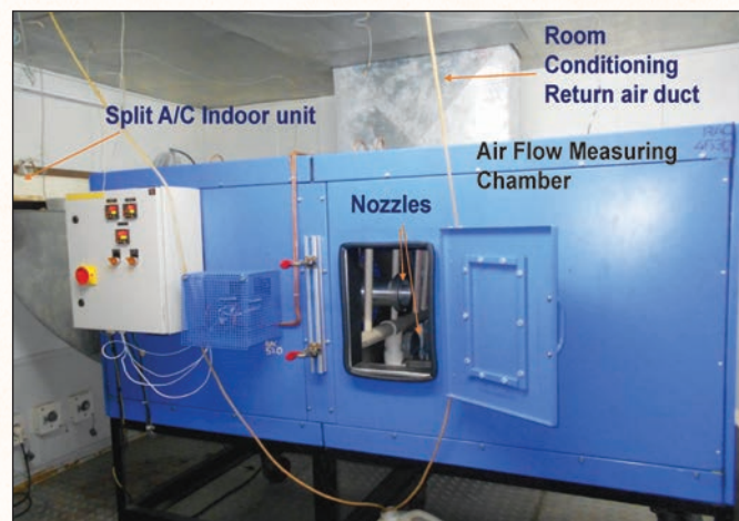
Figure 3: Photographic view of indoor room with air flow measuring chamber
