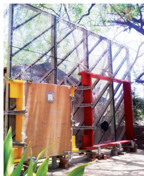
Photo 1: Air leakage chamber
