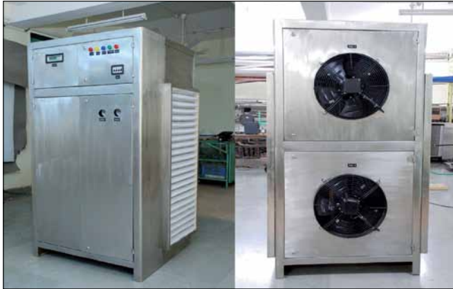
Figure 4: Multi-utility air to water heat pump, AW_HP installed at an automobile manufacturing unit of Mahindra and Mahindra at Kandivli, Mumbai.
