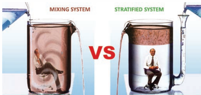
Figure 5: An under floor VAV system (right) provides improved occupant comfort versus a traditional overhead VAV system
