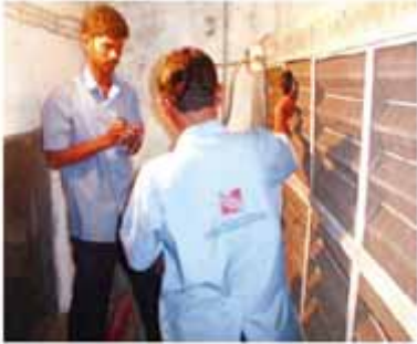
Measuring air flow after cleaning.
