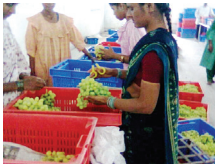
Photo 1: Packhouse maintained at 22°C & 75% RH for sorting, grading and packing.
