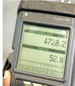
Figure 9: Ultrasonic water flow meter
