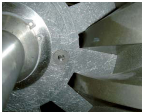
Figure 2. High pressure single screw rotors
