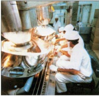
Dust containment on a bottle filling machine for tablet packing. Photo courtesy of Glaxo India Ltd.
