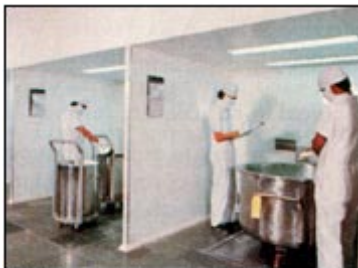
Weighing and dispensing booth for tablet bulk material and actives. Photo Courtesy of Glaxo India Ltd.
