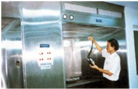
Reverse flow laminar dust containment booth with active dispensing table. Photo courtesy of Teknopak, Mumbai
