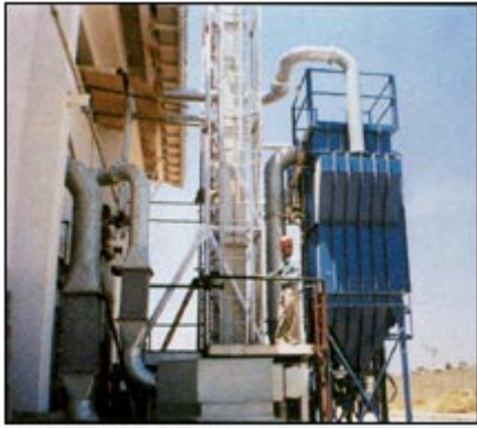
Bag type dust collector Photo courtesy of Laxmi Air Control Ltd., Mumbai
