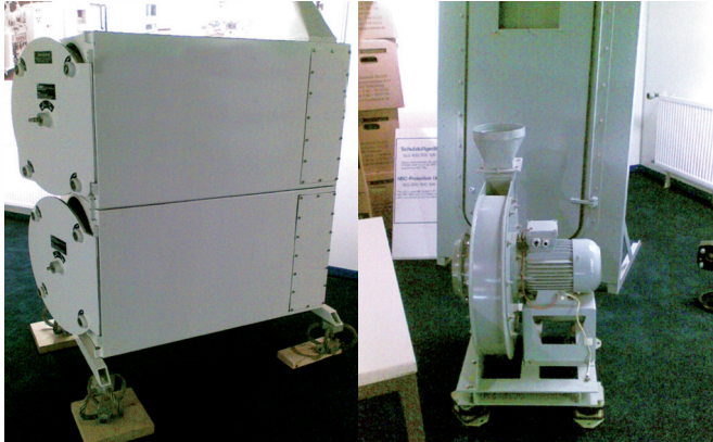
Figure 5: NBC filtration unit and AFU fan
