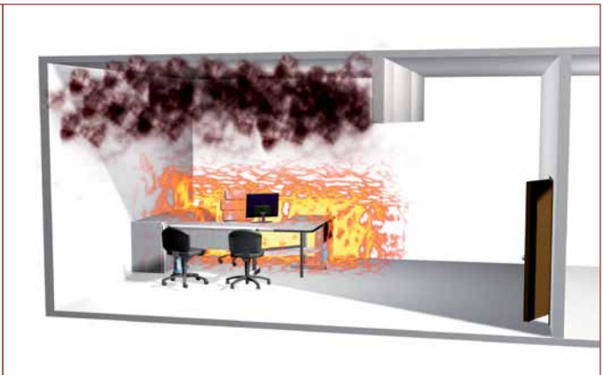
Figure 2 above and Figure 3 alongside show the effects of employing smoke curtains to act as a smoke reservoir.
