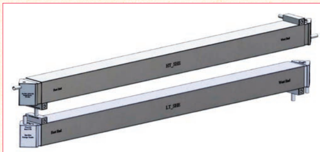
Figure 2: High and low temperature solution heat exchangers
