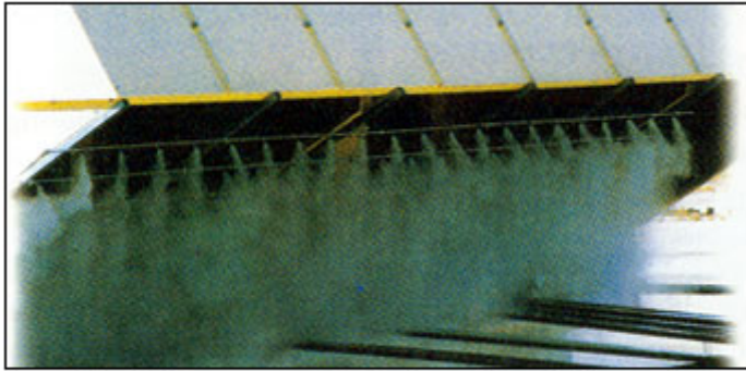
Fig. 1 Tube array containing impact pin fog nozzles
