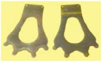
Figure 4c : Impressions of ports on valve plate due to deformation.
