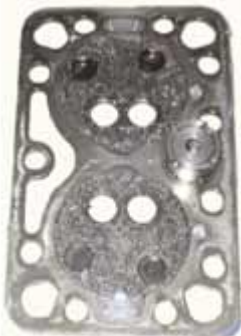
Figure 4a : Sludge and carbon deposits on valve plate.
