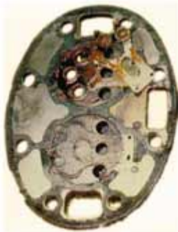
Figure 5 : Oily/Sludge valve plate.
