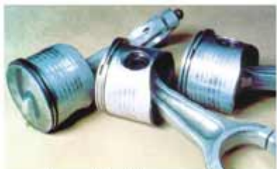
Figure 11a : Worn out pistons.
