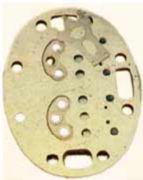
Figure 6 : Dry valve plate.
