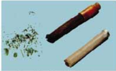
Figure 12a : Choked oil strainer.
