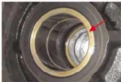
Figure 13 : Bearing surface turned reddish.
