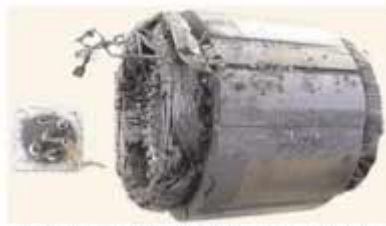
Figure 17a : Electrical motor stator failure.
