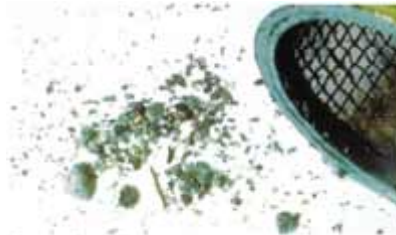
Figure 12b : Choked compressor suction strainer.
