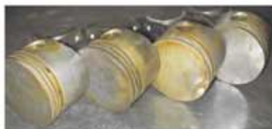
Figure 11b : Piston overheating.
