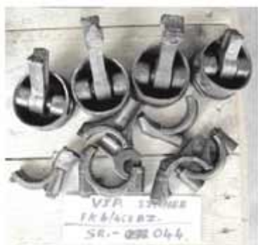
Figure 10a : Broken connecting rods.
