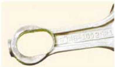
Figure 9 : Oblong small end of the connecting rod.
