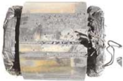
Figure 17 : Motor failure due to contaminants.
