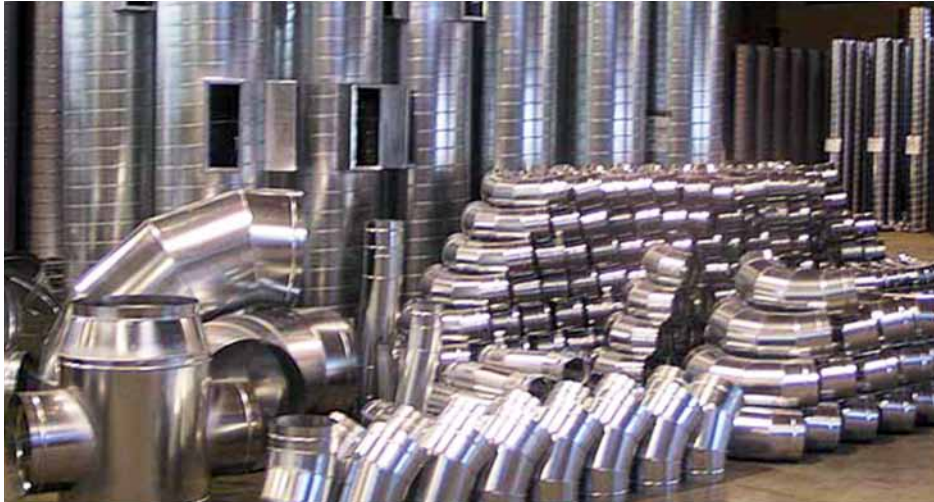
Photo 8: Pre-fabricated spiral ducts
