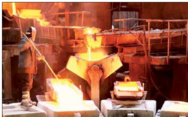
Molten copper being drained out from a smelter
