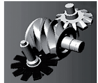
Figure 2 : Single screw rotor
