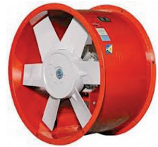
Figure 5: Fire rated axial fan (typically rated for 300°C, for 2 hours)
