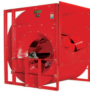
Figure 4: Fire rated centrifugal fan (typically rated for 300°C, for 2 hours)
