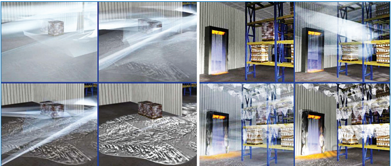
Figure 5-3: Excessive ice in cold storage due to ineffective vapour barrier
