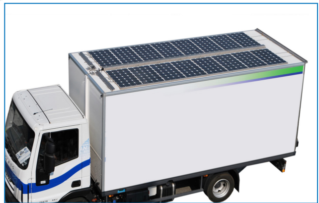
Figure 8-11: A solar powered refrigerated truck
