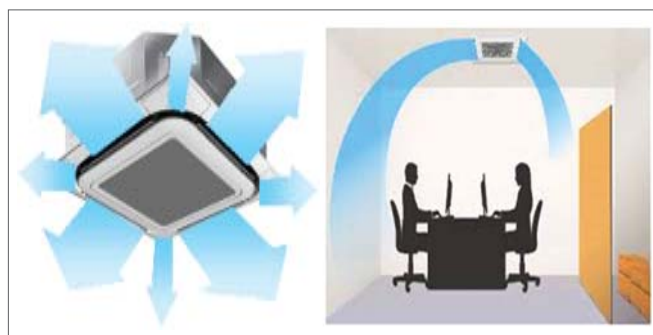
Figure 5: Air flow from a cassette unit
