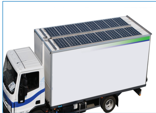
Figure 8-11: A solar powered refrigerated truck
