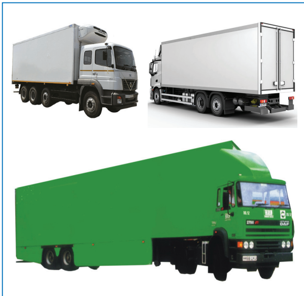
Figure 8-4: Trucks with PUF panels
