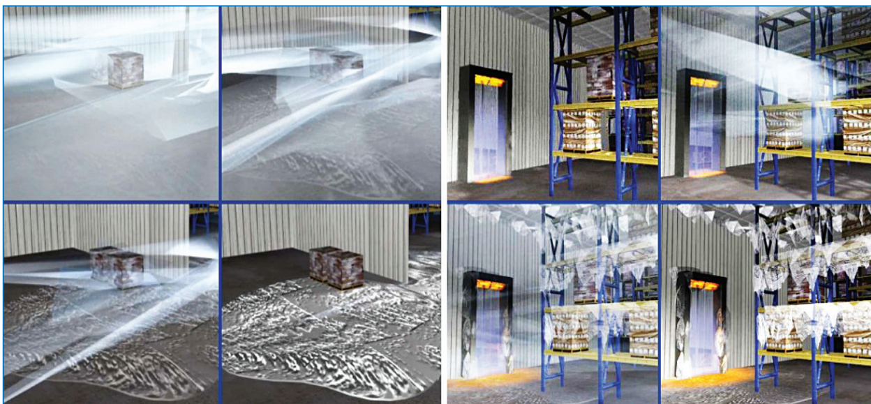
Figure 5-3: Excessive ice in cold storage due to ineffective vapour barrier
