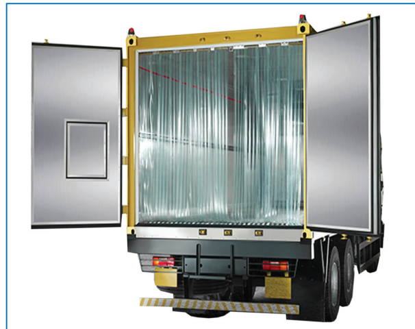
Figure 8-18: PVC curtain behind the door to reduce heat gain from outside air
