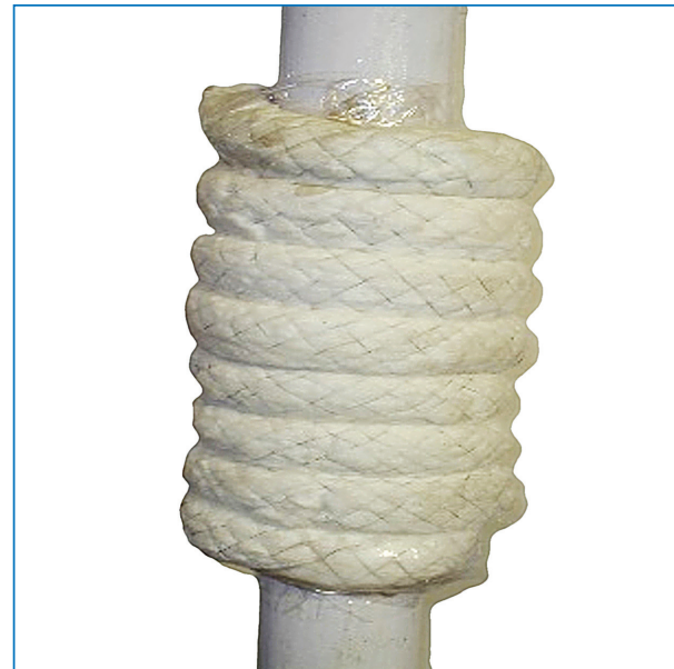
Figure 6-10: Rope wound around a small pipe
