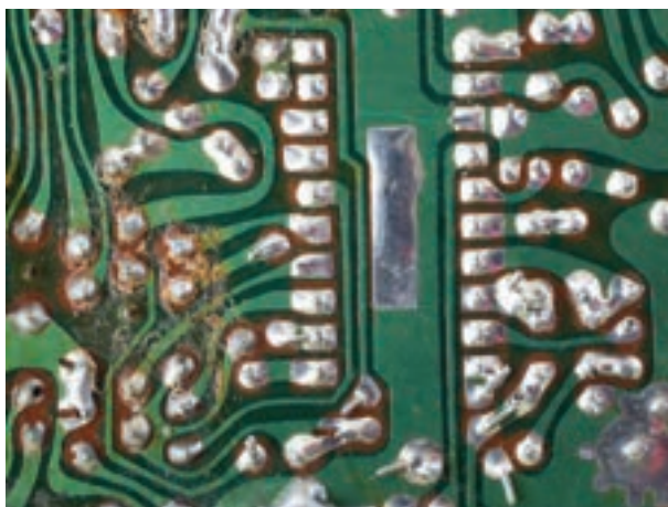
Figure 20.4: Corrosion on electronic parts
