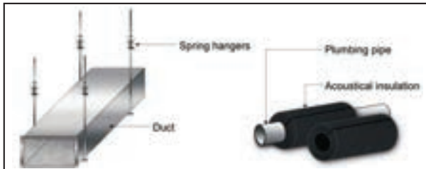
Figure 18.5: Isolating ducts and pipes
