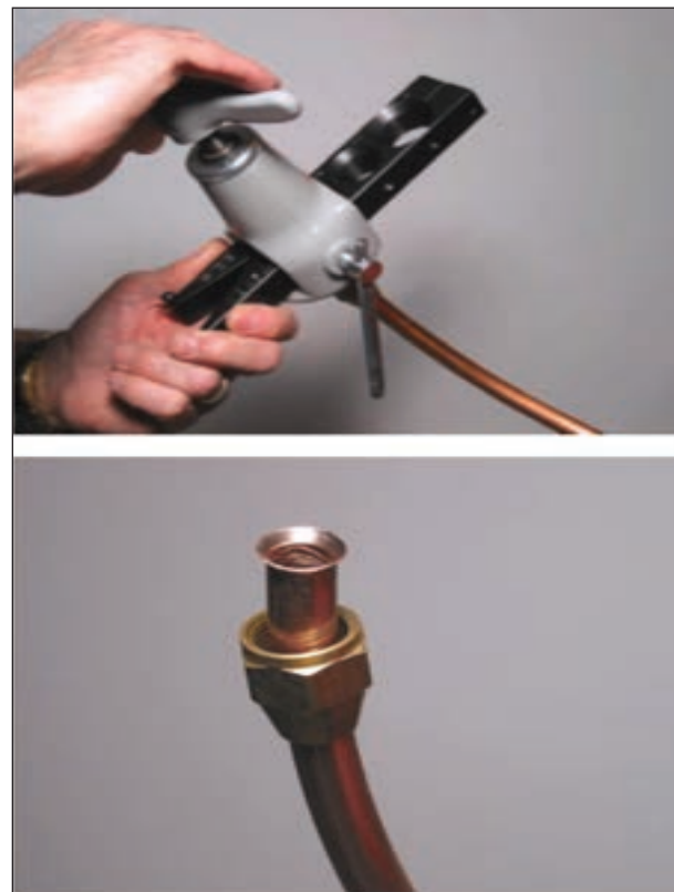
Figure 3.16: (a) Lowering the flaring cone into the tube end (b) Completed flared tube
