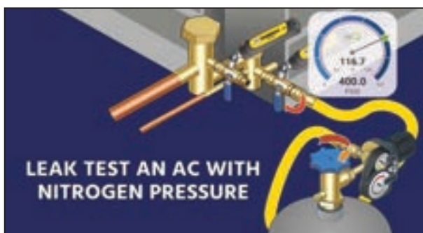
Figure 21.4: Pressure testing of refrigerant piping
