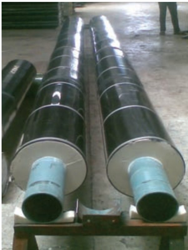
Figure 13.2: Pre insulated pipe with HDPE cladding
