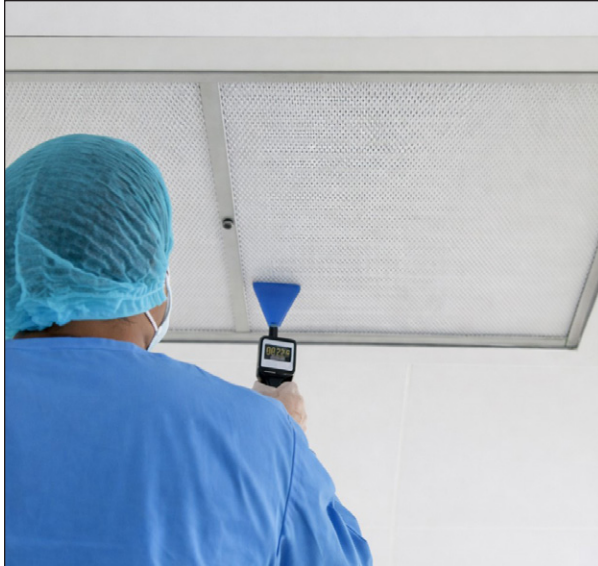
Figure 5: HEPA filter Test Scanning with Photometer
