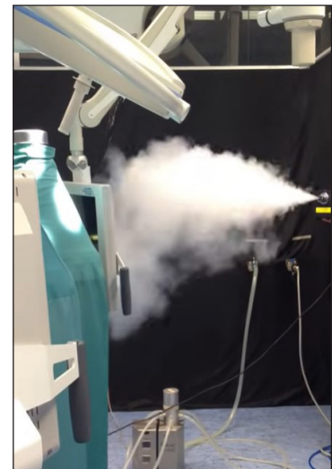
Figure 9: Air Flow Pattern Test in an Operation Theatre
